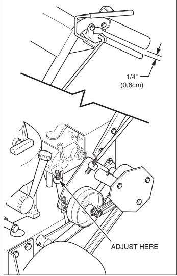
Figure 11. Brake Adjustment
